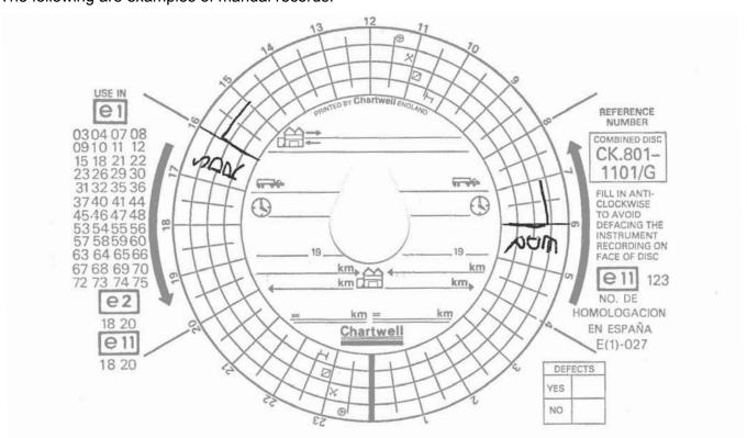
This is an example of manual entries made on the rear of a tachograph chart of a driver who started his day at 06.00 with an hour's work doing other duties away from his vehicle. He also finished his day with an hour of other work away from his vehicle and has indicated both the end and the start of a daily rest period. His activities while with the vehicle are recorded by the instrument on the other side of the chart once it has been inserted.
